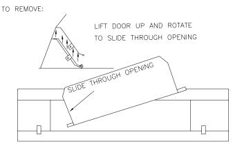
FIGURE 11a: DAMPER DOOR REMOVAL
